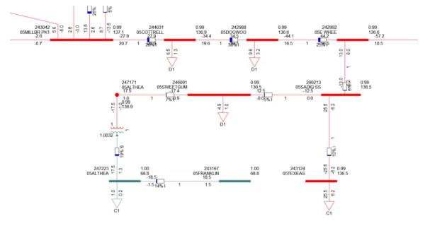
Figure 3-4. System with proposed facility, N-1 loss of Fuller – Argentum (EKPC) 138 kV line
