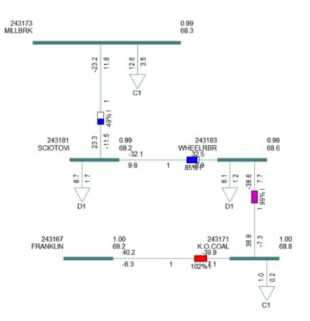
Figure 3-2. System without proposed facility, N-1 loss of Fuller-Argentum (EKPC) 138 kV line.
